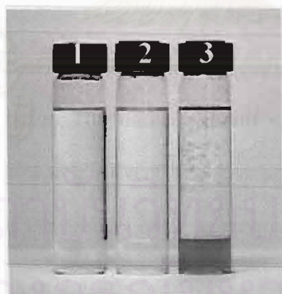
Figure 4-66 The color of extracted lower phase of hexyl-3-aminobenzoate azo dyes having substituent group as 2-chloro-4-nitro group.
