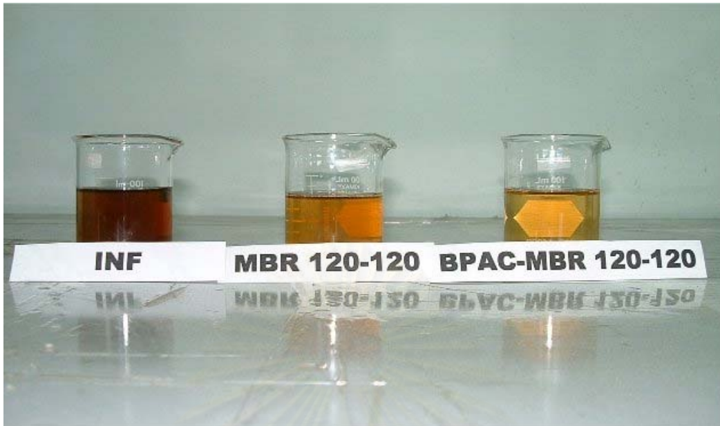
Figure 4.41 Influent and effluent color of MBR and BPAC-MBR at an intermittent aeration time of 120-120 minutes
