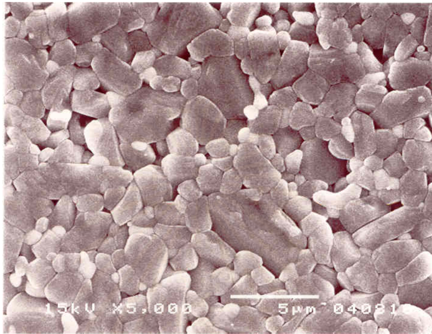
Fig. 4.11(a) SEM micrograph of 6% SPZ added specimen (KM04), sintered at 1650°C
