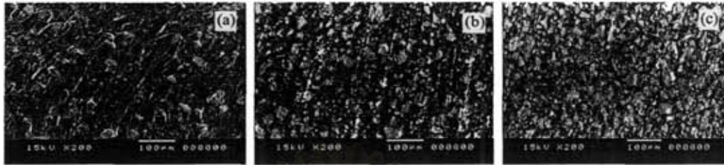
Figure 2 SEM micrographs of the composites with (a) 30 wt%, (b) 50 wt%, and (c) 80 wt% of BST
