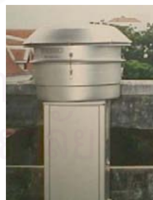
Figure 3.9 High volume air sampler attached with PM10 inlet
