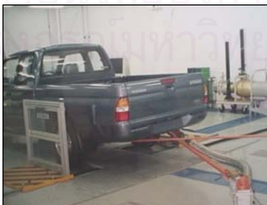
Figure 3.14 LDDV emission test
