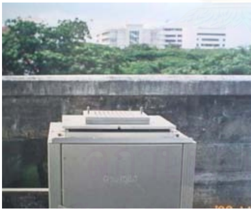
Figure 3.10 High volume air sampler attached with SFPM impactor
