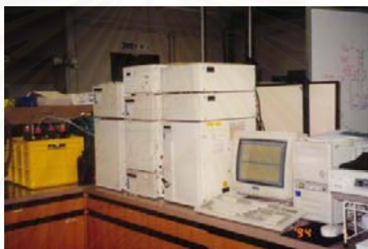
Figure 3.17 High Performance Liquid Chromatography Shimazu LC-10 HPLC Model CBM-10A
