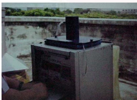
Figure 3.8 Calibration of high volume sampler
