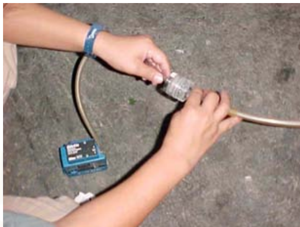
Figure 3.20 Gasoline vehicles sampling Figure 3.21 Low flow pump and PVC cassette
