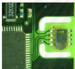
Figure 8 SHT1x Mounting example
