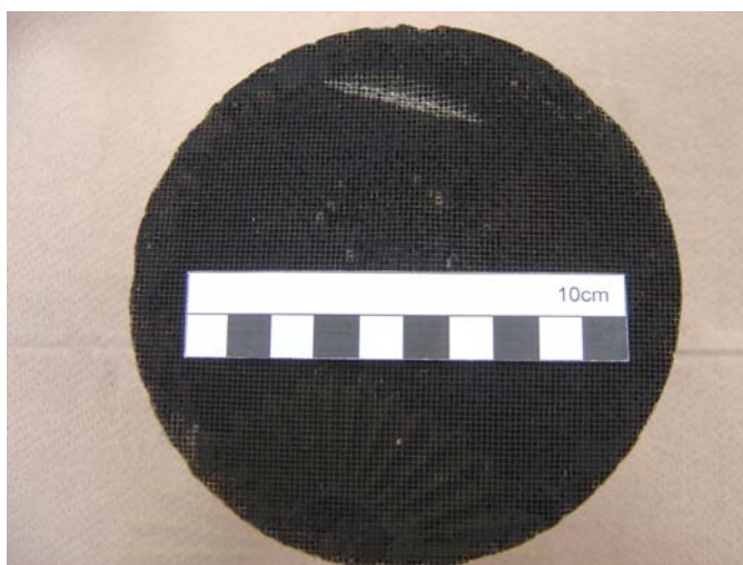
Figure 2.3 Cross section of spent automobile catalytic converter used in this present study
