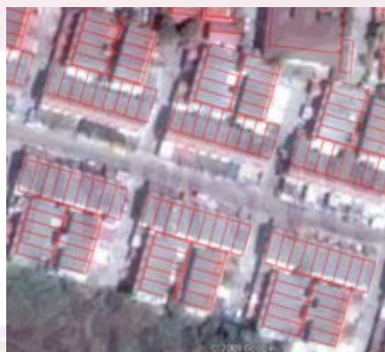
Figure 4.30 The file after warpping and comparing with the orthophoto from Google Earth.
