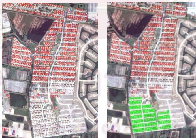
Figure 4.34 The left picture is before update. The right one is after digitizing houses.
