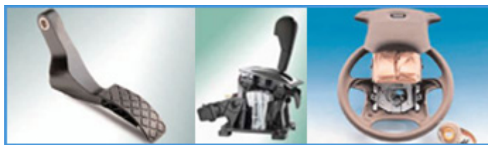
Figure 2.3 Examples of Applications, such as Pedals, Gear Shift Console, Airbag Canister Housings [3]
