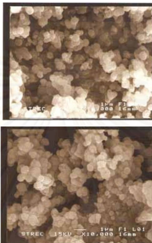
Figure 5.31 SEM micrograph for the NiTiSSP550 and NiTiSSP650 catalysts.
