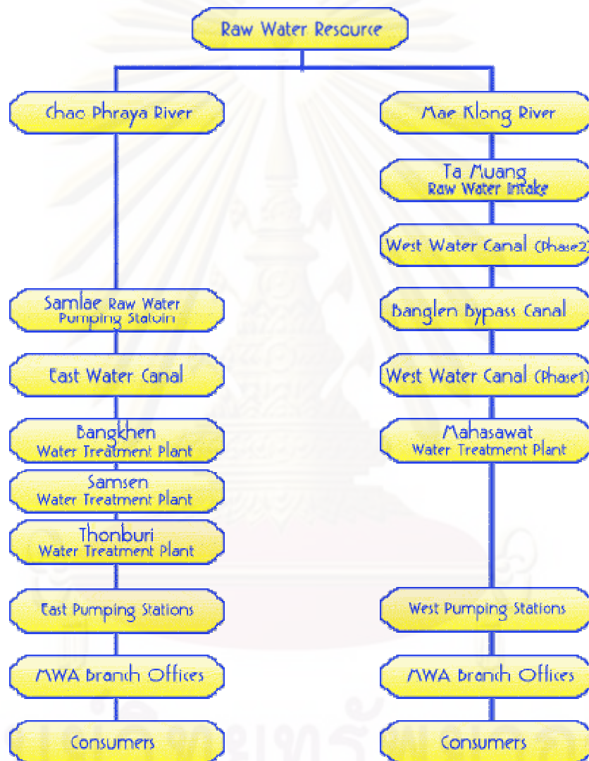
Figure 2.8 Diagram of water resources and their transmission to consumers.
