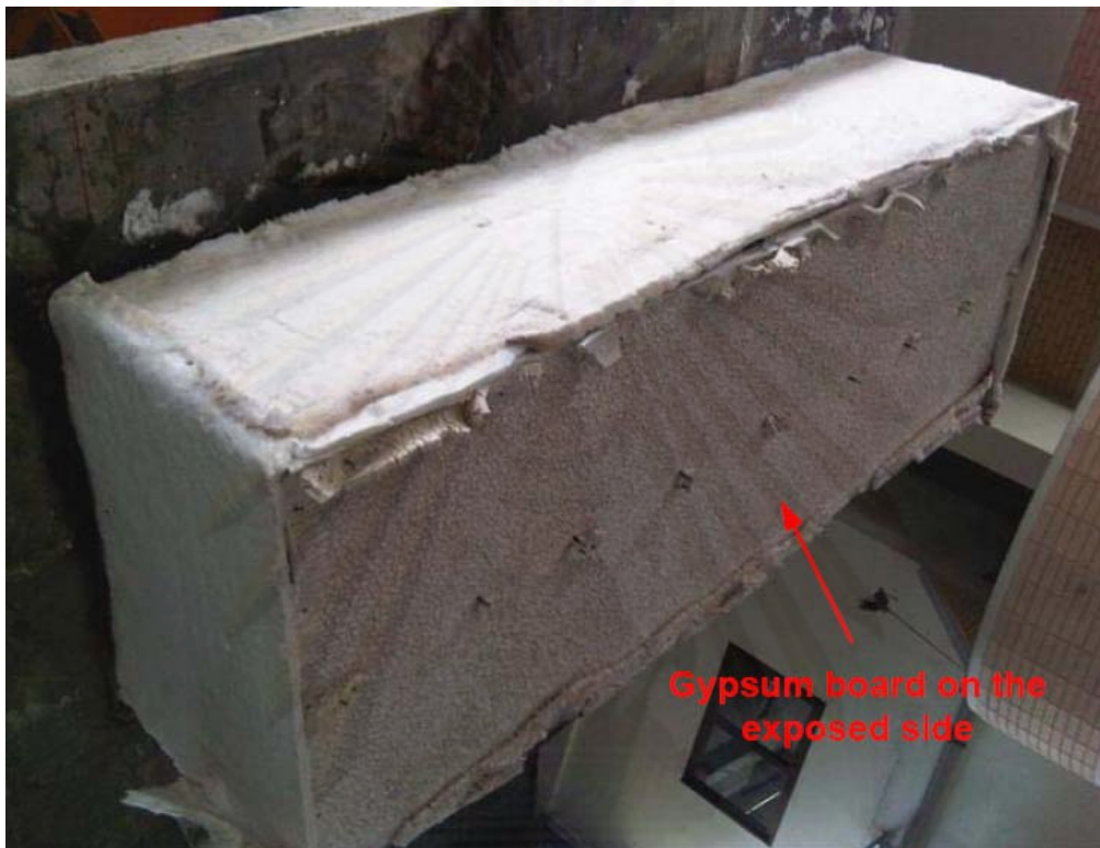
Figure 4.24 Specimen-3 after the fire test
