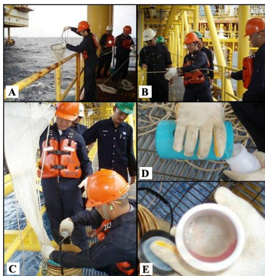
Figure 3.4 Plankton sampling at experimental sites. Planktons were collected using 20 micron mesh (A, B, and C). Collected planktons were preserved in plastic bottle containing 3% neutral formaldehyde (D and E).
