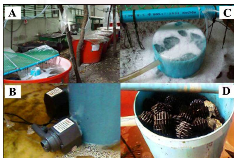
Figure 4.10 Experiment tanks for rearing of green mussels (A) and details of bioreactor used for nitrogenous waste treatment (B, C, and D).
