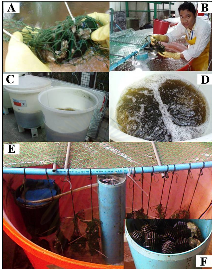
Figure 3.1 Green Mussel tanks maintained in Laboratory. mussel bag (A), worker (B), plankton culture tank (C and D), mussel tank show bioreactor (E), enlarge bioreactor (F)
