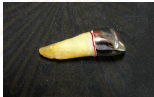
Fig. 11 Fracture mode of specimen which was horizontal root fracture at cervical of root
