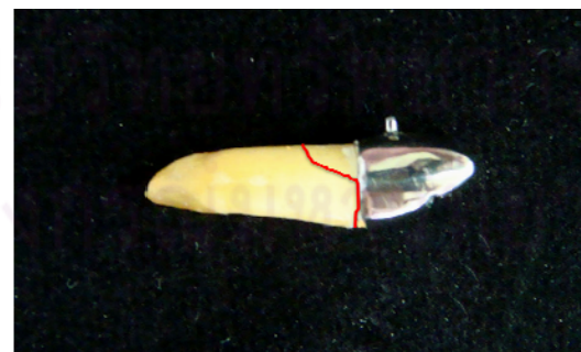
Fig. 13 Fracture mode of specimen which was debonding of margin combined with cervical root fracture
