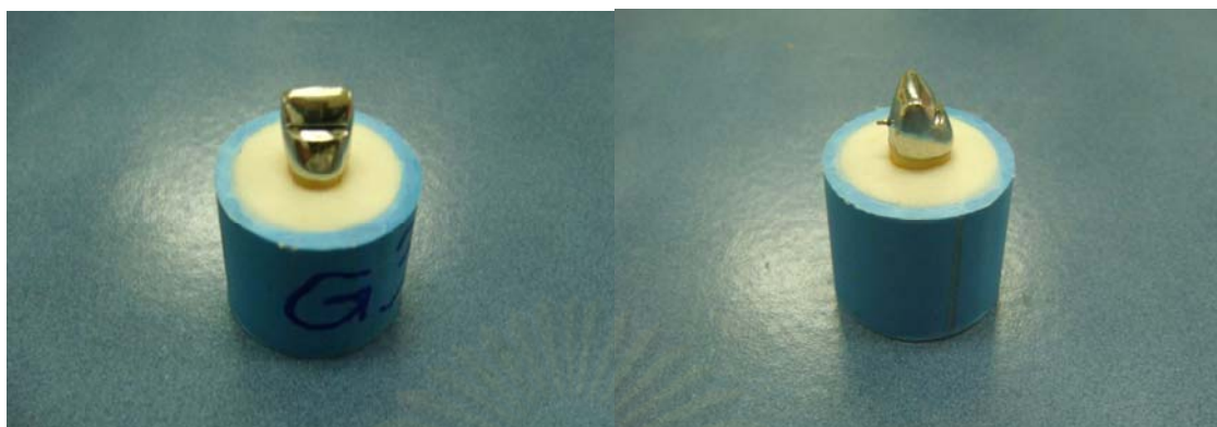
Fig. 8 Specimen for fracture resistance test
