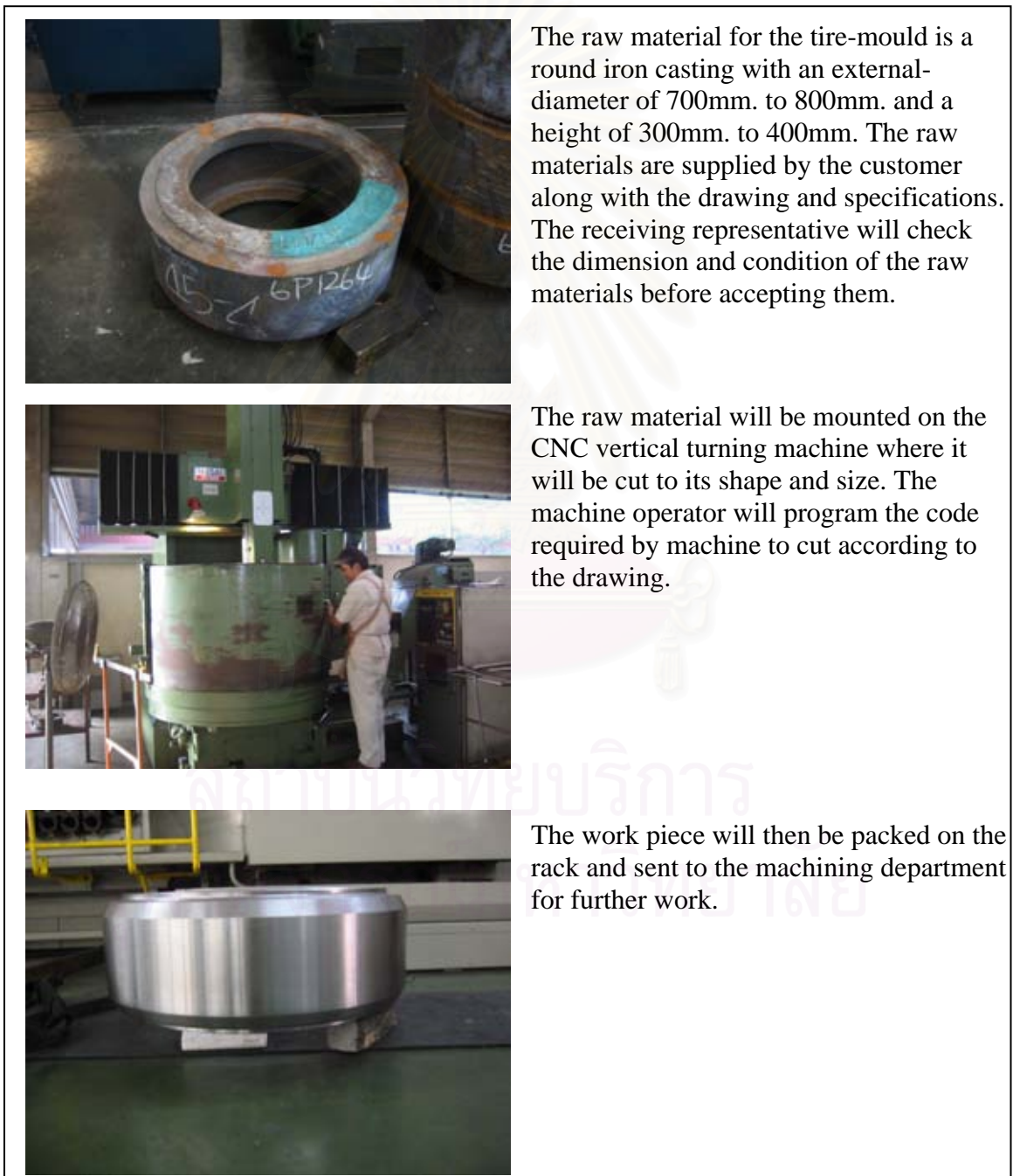
Figure 3.2 : Tire Mould Production Process
