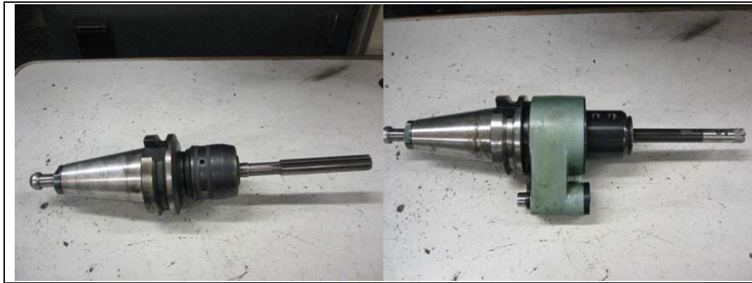
Figure 5.2 : High-speed reamer (left), Carbide reamer (right)
