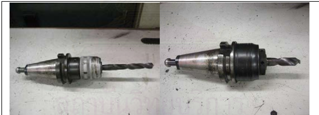
Figure 5.1 : High-speed drill (left), Carbide drill (right)
