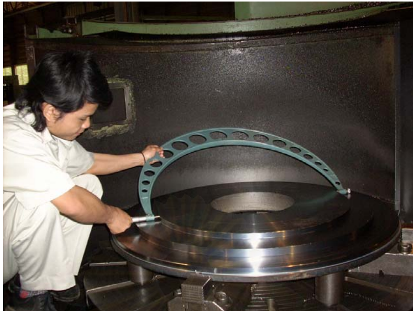
Figure 6.6 : Operator Checking the Dimension
