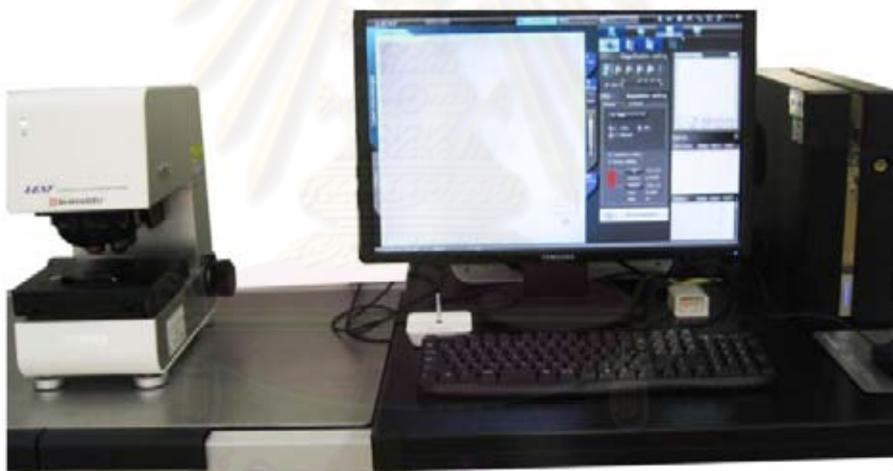
**Figure 2.6** Confocal Laser Microscope
