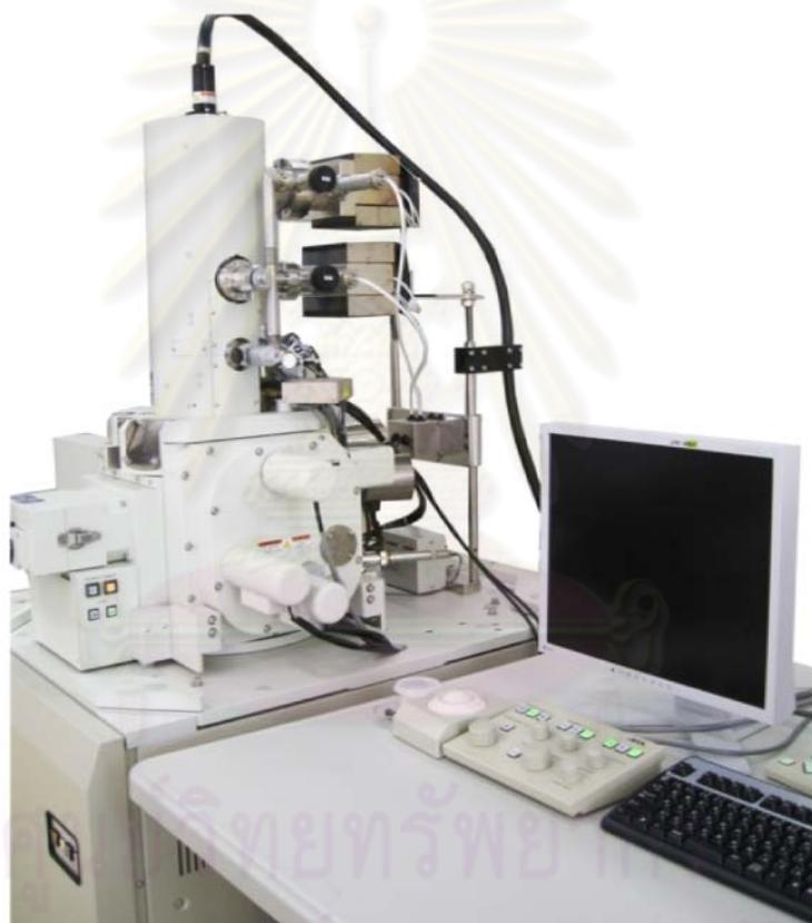
**Figure 2.8** Field Emission Scanning Electron Microscope (FE-SEM; JSM7600F; JEOL)
