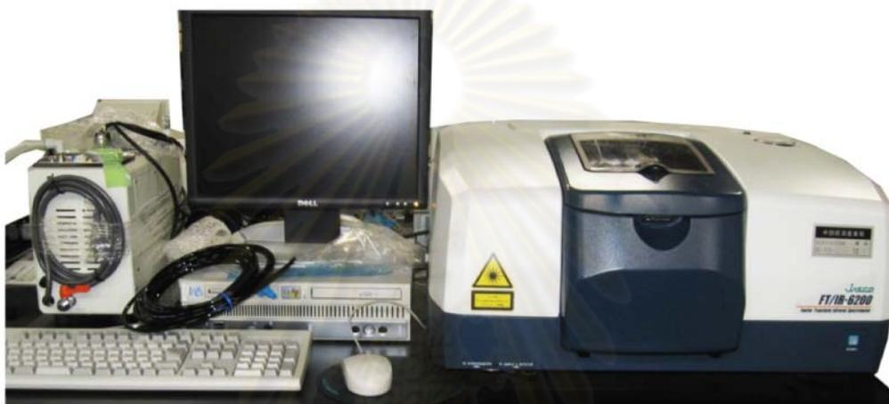
**Figure 2.7** Fourier transform infrared spectroscopy (FTIR; FT/IR6200 JASCO)
