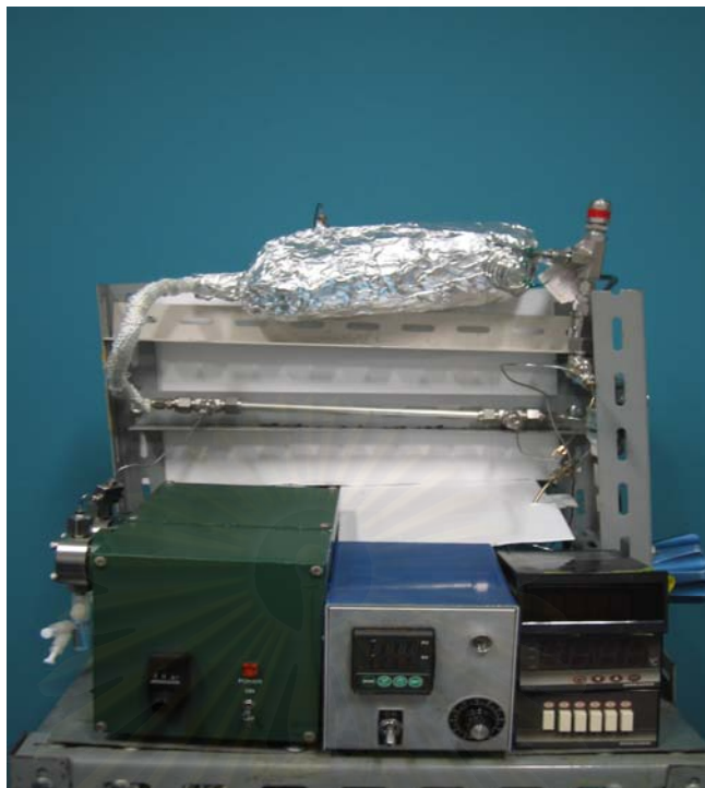
Figure 3.3 Catalytic SCWO compact sized reactor for laboratory waste treatment
