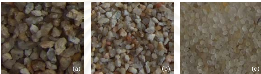
Figure 3-1 Shape of grain particle of (a) D16, (b) D40 and (c) Silica test sand.
