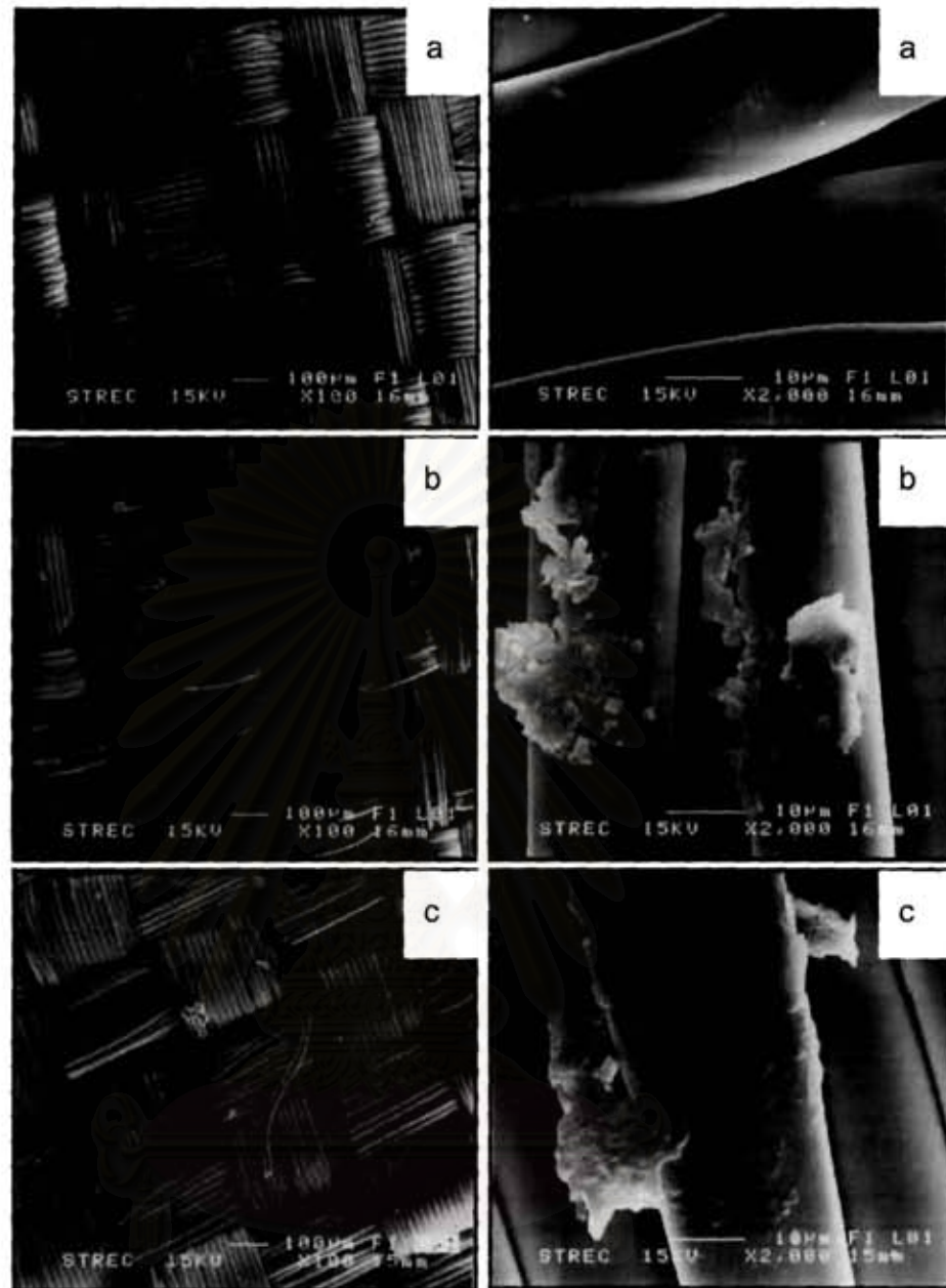
Figure 4.11 SEM photographs at X100 (left) and X2000 (right) of untreated nylon 6 fabric (a), nylon 6 fabrics treated with 20 (b), and 40 (c) shots of nitrogen plasma
