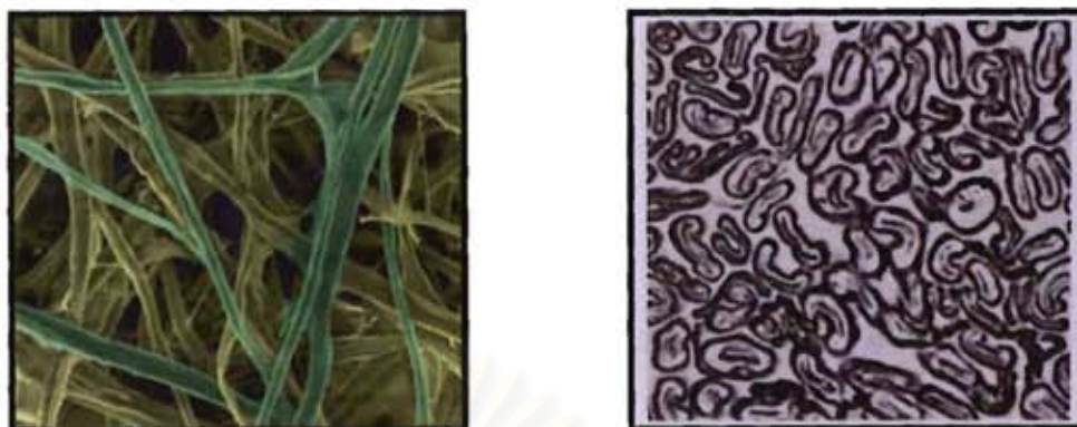
Figure 2.4 SEM and optical photographs of raw cotton fiber in a cross section (right) and a longitudinal view (left) [16].
