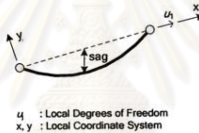
Figure 2.3 Cable element with sag
