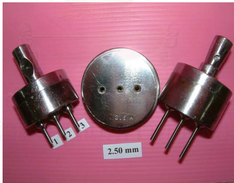
Figure 11 Special punches and dies of 2.50 mm diameter
