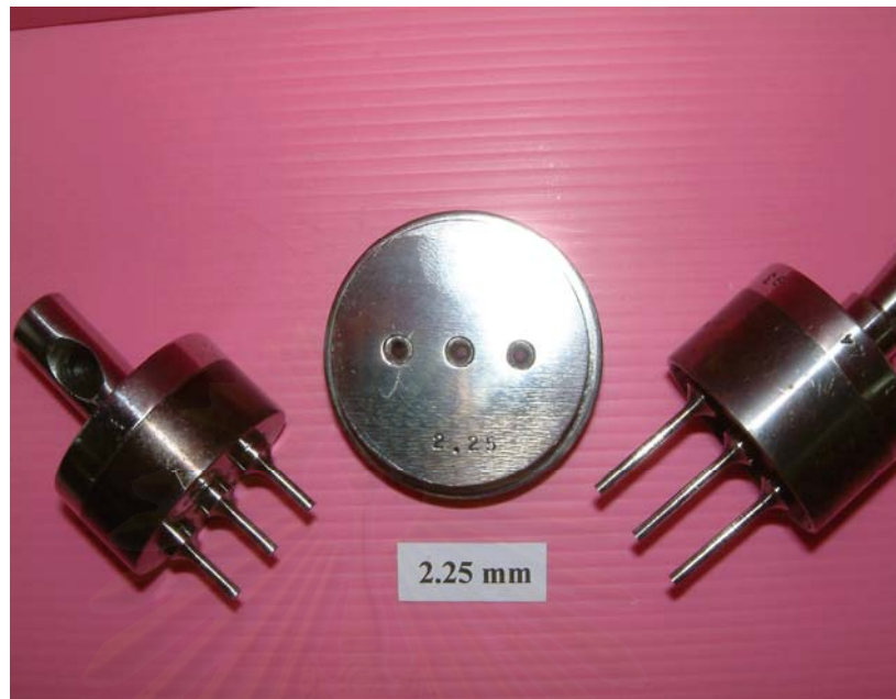
Figure 10 Special punches and dies of 2.25 mm diameter
