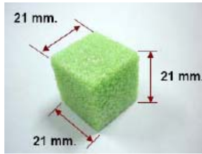
Figure 3.13 A cube specimen prepared
