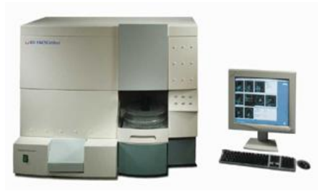
Figure 3.3 The feature of BD FACScalibur™ flow cytometer used for Flow cytometric quantitative analysis in this study (from Becton and Dickinson, USA).
