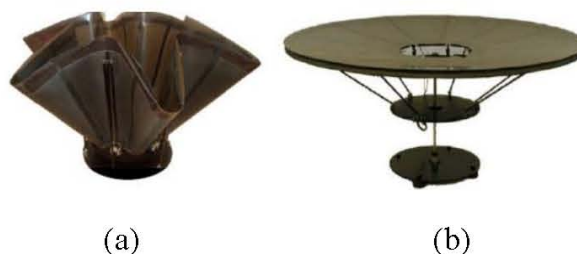
Figure 2.11 Shape memory polymer composite reflectors: (a) pre-deformed shape and (b) recovered shape (Leng et al., 2011).
