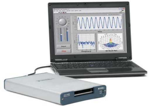
Fig. 6 A DAQ based arbitrary waveform generator
