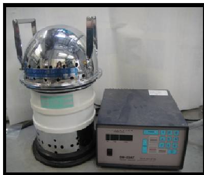
Figure 4.17 Ultrasonic single sieving
