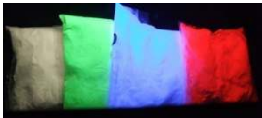
Figure 3.1 Fresh samples in 325 \mu\text{m} wave length light (white, red, blue and green phosphor)
