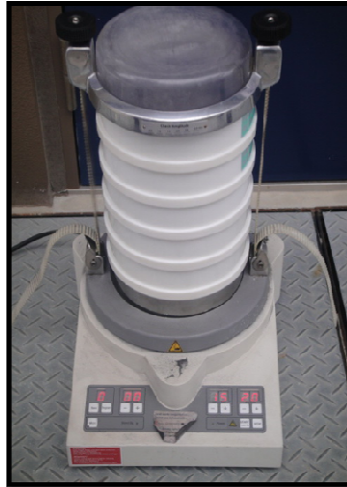
Figure 4.1 Vibration sieving machine and sieve opening 20, 16, 12.5, 10, 8 and 5 \mu\text{m}
