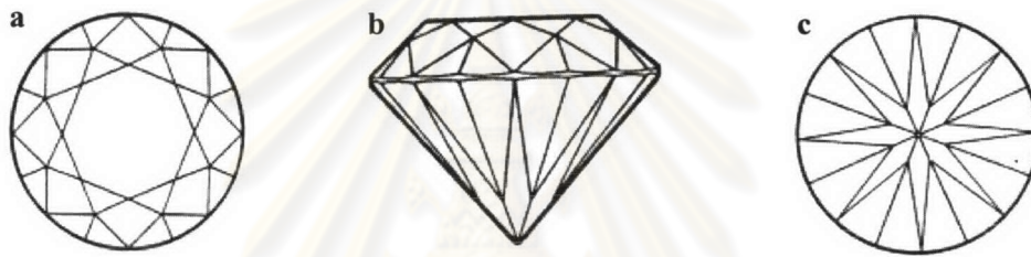
Figure 2.7 Popular diamond cuts. The picture shows three different views of the brilliant cut, with 57 facets. a , crown with 32 facets, plus the large table facet; b , side view; and c , pavilion with 16 lower girdle and 8 pavilion facets. If there is a culet facet, the total will be 58 facets.
