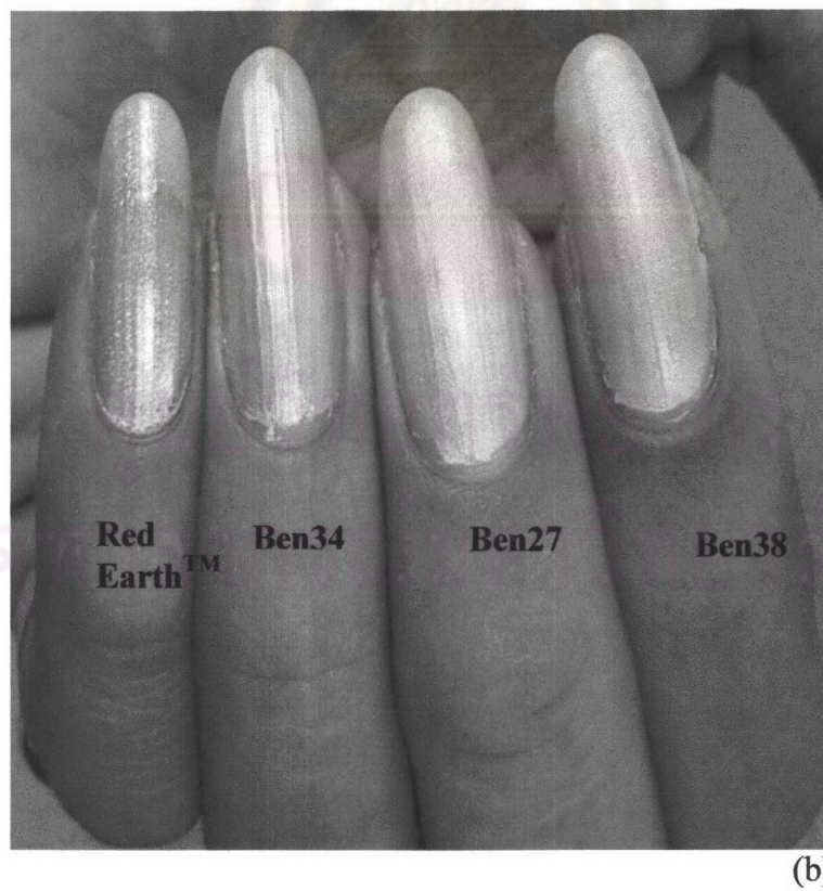
Figure 5.26 Comparative test on human of formulated nail enamels of various suspending agents: (a) 1 day (b) 10 days
