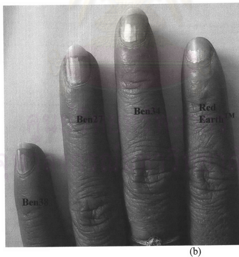
Figure 5.27 Comparative test on human of formulated nail enamels of various suspending agents: (a) 1 day (b) 10 days
