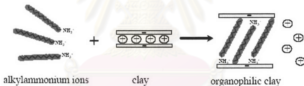
Figure 2.6 The cation-exchange process between alkylammonium ions and cations initially intercalated between clay layers [10]
