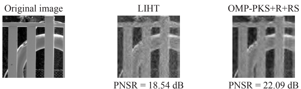
Figure 4.47: The part of reconstructed Fence based on LIHT and OMP-PKS+R+RS when \mathbf{y} is corrupted by Gaussian and impulsive noise at M/N = 0.3 , \sigma^2 = 0.1 and q = 0.05 .
