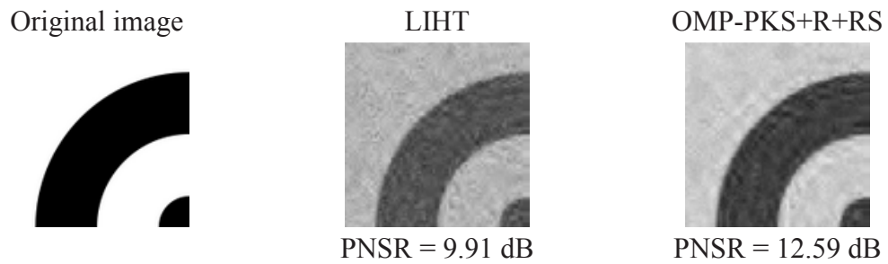
Figure 4.45: The part of reconstructed Arc based on LIHT and OMP-PKS+R+RS when \mathbf{y} is corrupted by Gaussian and impulsive noise at M/N = 0.3 , \sigma^2 = 0.1 and q = 0.05 .
