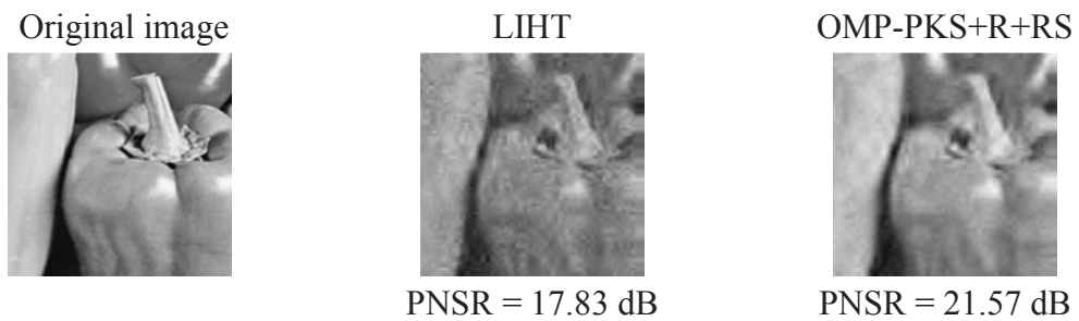
Figure 4.42: The part of reconstructed Peppers based on LIHT and OMP-PKS+R+RS when \mathbf{y} is corrupted by Gaussian and impulsive noise at M/N = 0.3 , \sigma^2 = 0.1 and q = 0.05 .
