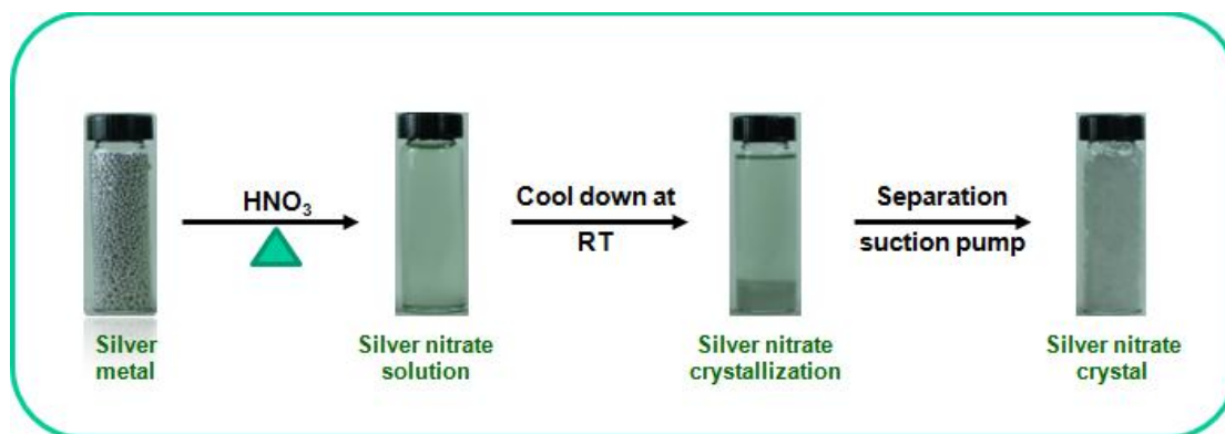
Figure 3.1 Schematic synthesis method of silver nitrate.
