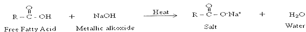
Figure 2.5 Saponification reaction of the produced fatty acid alkyl esters. (Schuchhardt et al., 1997)
