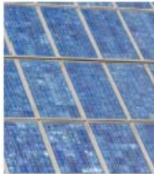
Figure 1.5 Multicrystalline silicon PV panel
