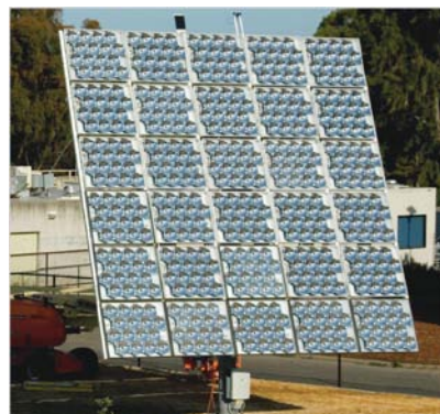
Figure 1.9 Concentrated photovoltaic system
