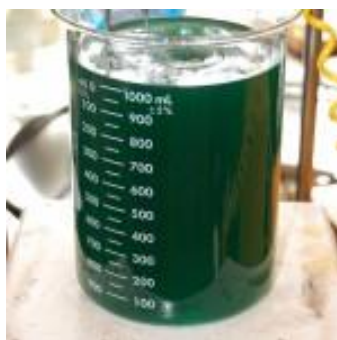
Figure 2.1 Electroless nickel plating solution [15].
