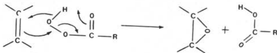
Figure.44 Mechanism of epoxidation of m -chloroperbenzoic acid.
