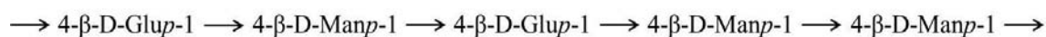
Figure 1.7 Simplified structural formula of hardwoods hemicellulose glucomannan [38, 40]. Sugar units: Glup (Glucopyranose); Manp (Mannopyranose).
