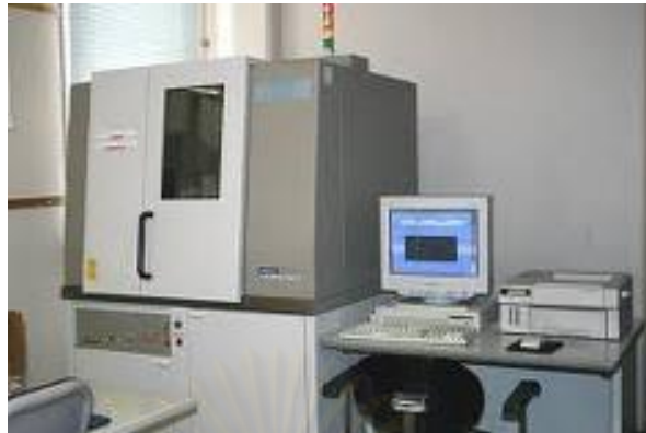
Figure 3.10 X-ray diffractometer (XRD), Rigaku Geigerflex X-ray diffractometer equipped with a CuK-radiation source.
