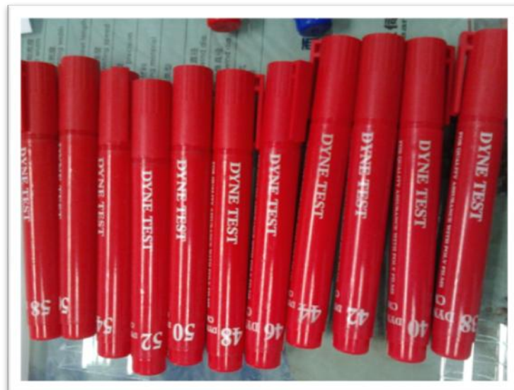
Figure 9. Poly-Test dyne pen solution number 38-58 dyne/cm for test surface energy on both of sample compostable plastics.
