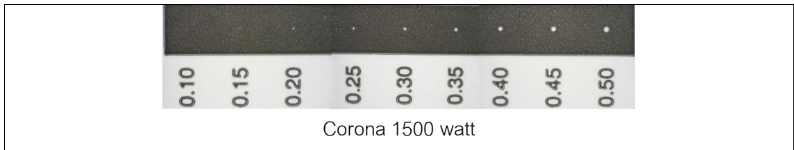
Figure 16. Negative micro dot tap on PLA/PBAT used anilox line resolution at 600 lpi
