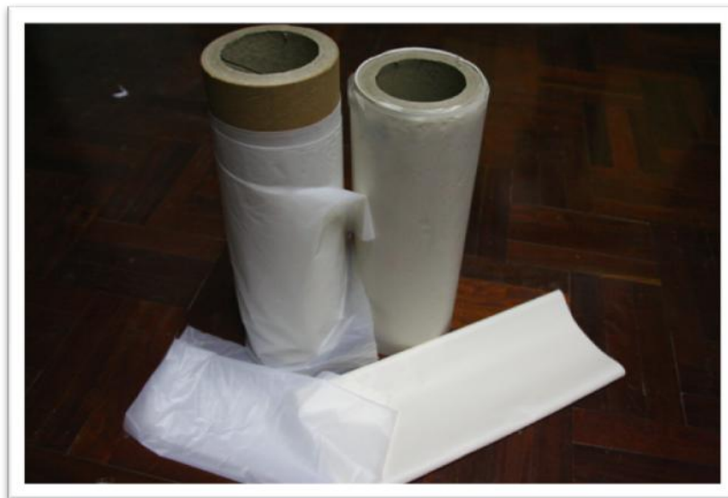
Figure 1. Sample compostable plastics film PBAT/Starch (left); 40 \mu\text{m} thickness and PLA/PBAT (right); 100 \mu\text{m} thickness substrate for printed in this experiment.
