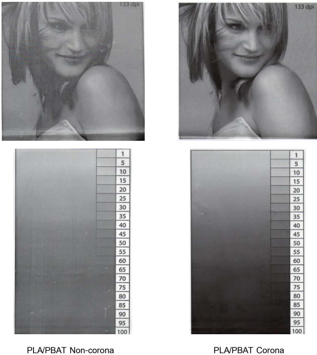
Figure 4-3 Examples image area printed on PLA/PBAT non-corona and corona treatment at 500 watt and used anilox line resolution at 700 lpi.
