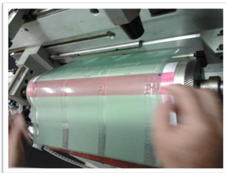
Figure 2. Photopolymer plate hardness 64°, shore A and 1.14 mm thickness from Flint group Co., Ltd.
