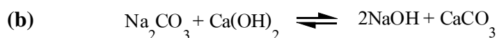
Scheme 2.2 A schematic of the manufacture of \text{CaCO}_3 by (a) \text{Na}_2\text{CO}_3 or (b) \text{NaOH} .
