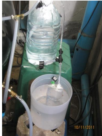
Figure 3.7 Water displacement method
