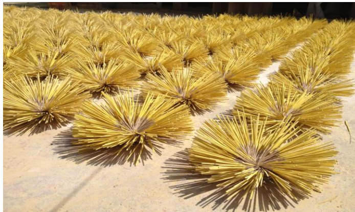
Figure 2.3 Molding and drying the upper part of incense stick
