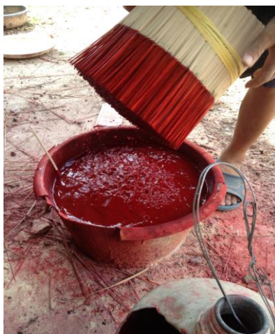
Figure 2.4 Dissolved dye for dipping the lower part of incense stick
