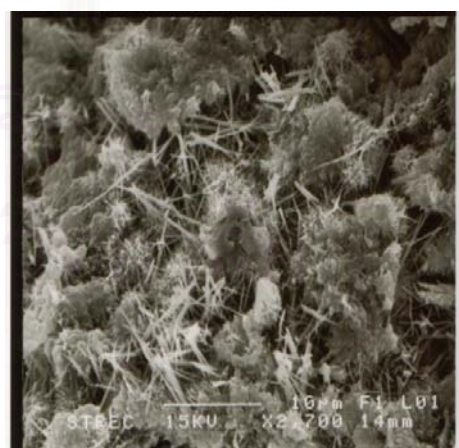
(f) CFA 5 at 90 days, 2700x
