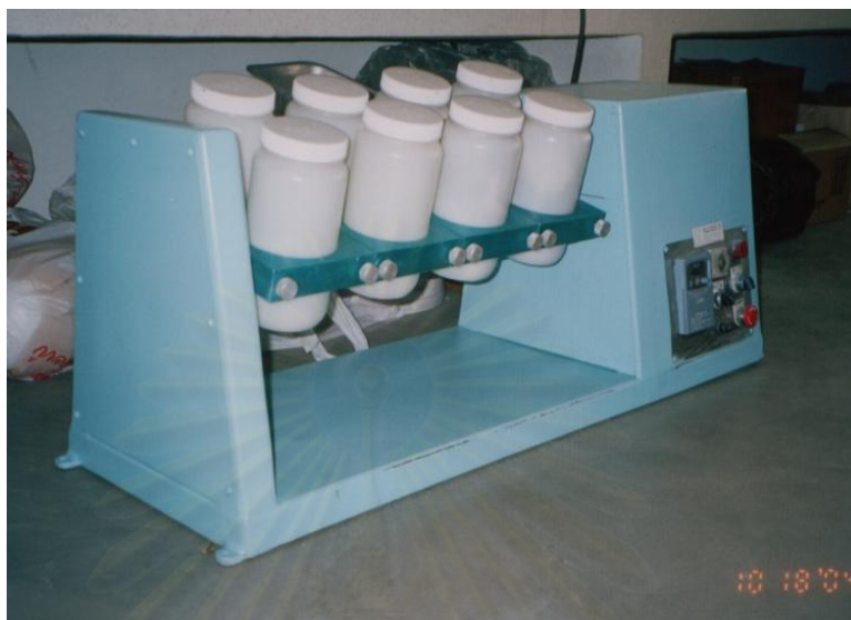
Figure A-5 Rotating Agitator for Leaching Test
