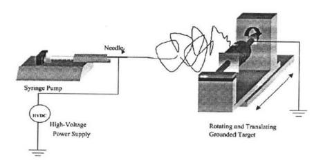
Figure 1.1 The electrospinning apparatus utilized in the production of ultrafine fibers.
