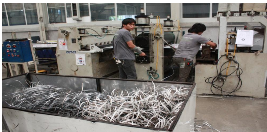
Figure 6.5 Operator cut edge of aluminium composite coil
