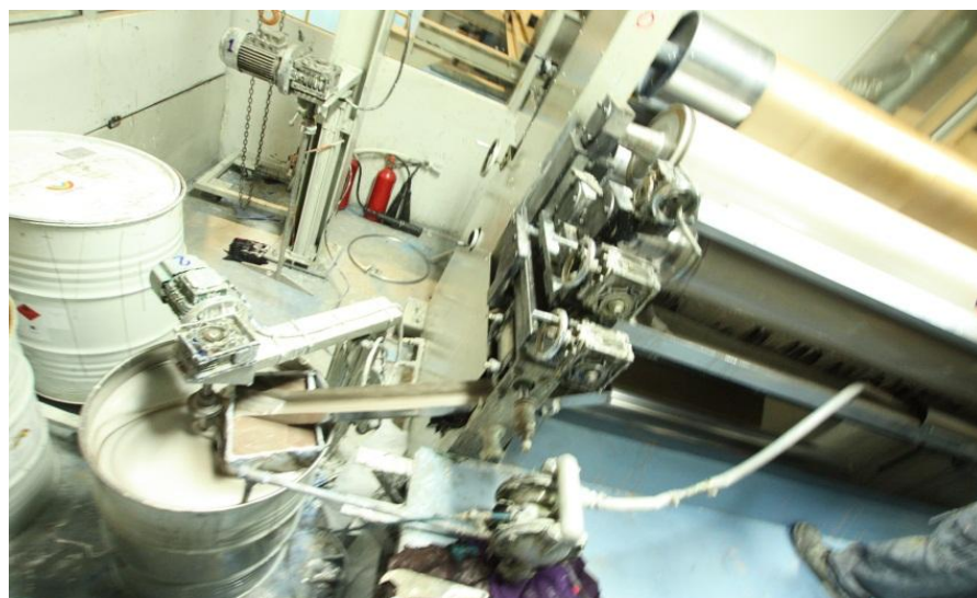
Figure 3.5 colour tank with screen filter and colour stirring motor
