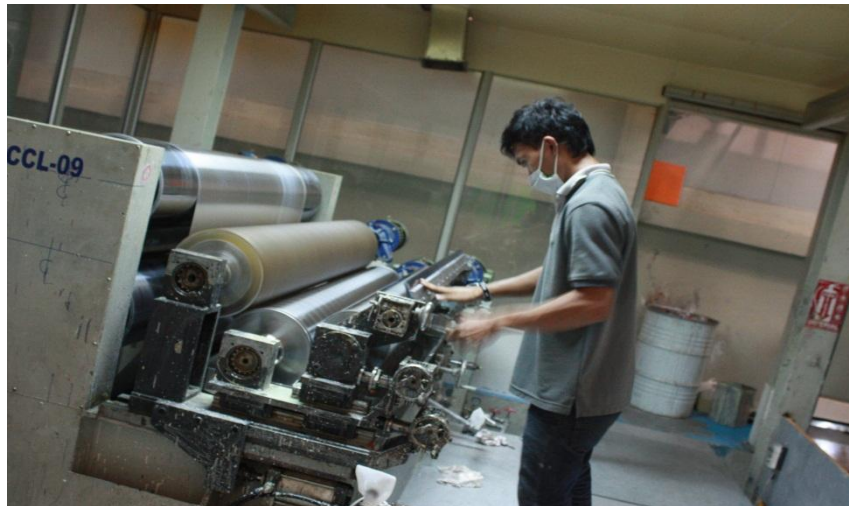
Figure 6.2 Operator is setting Scraper Roller
