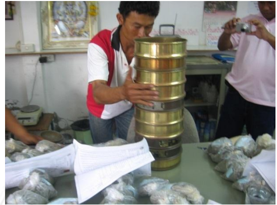
Figure 31 Sieve analysis of the sediment samples.
