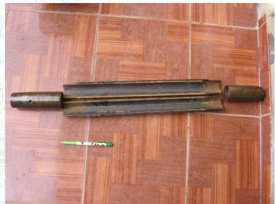
Figure 32 Drilling head of the lighter type (Motorind Cathead)
