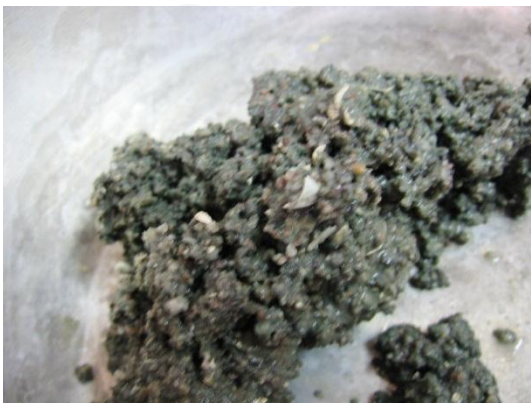
Figure 35 Offshore sandy mud in a deep layer of the borehole
