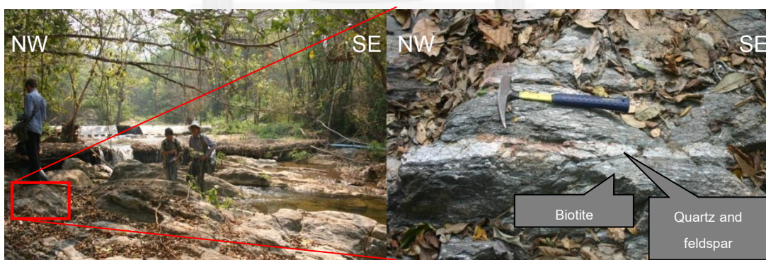
Figure 4. 2 (Left) an outcrop of rock sample location number LS-4. (Right) rock sample number LS- 4 presents dominant feature of porphyroblastic texture of quartz and feldspar in biotite.
