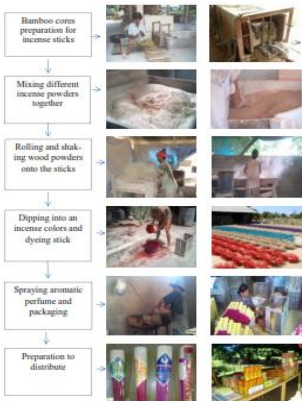
Figure 12 The process of incense stick making, “Toop Saad” method
