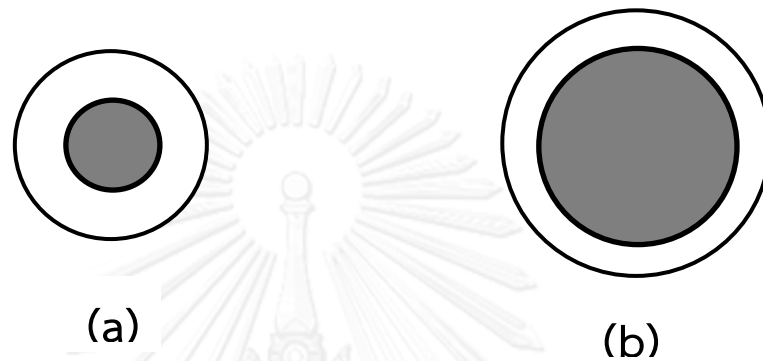
Figure 4-10. Schematic showing effect of core diameter on overall fiber diameter (a) smaller core diameter and larger sheath thickness, (b) larger core diameter and smaller sheath thickness [29].
