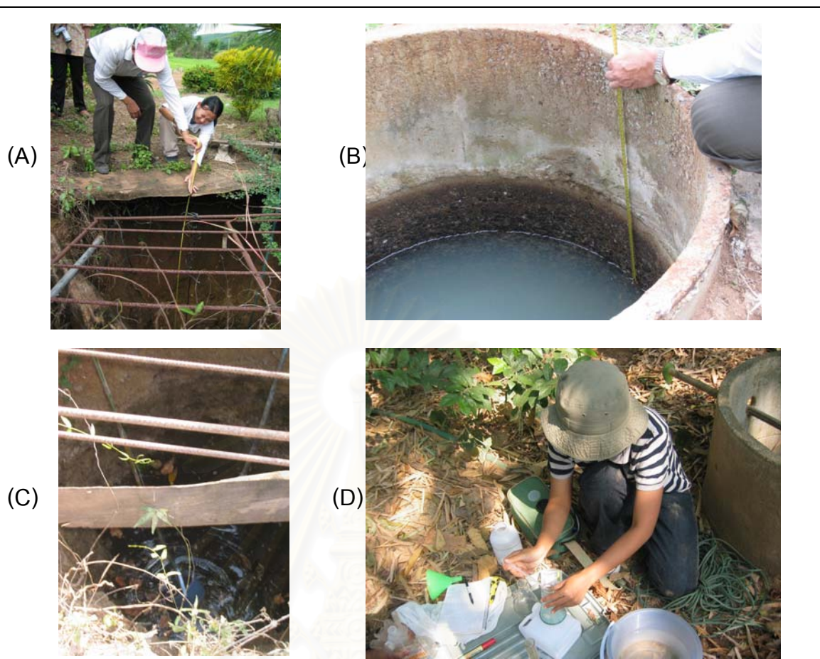
Figure 3.3. Field investigation of the shallow, unconfined groundwater. (A) and (B), Water table measurement , (C) and (D) Water sampling and field test for some chemical quality.
