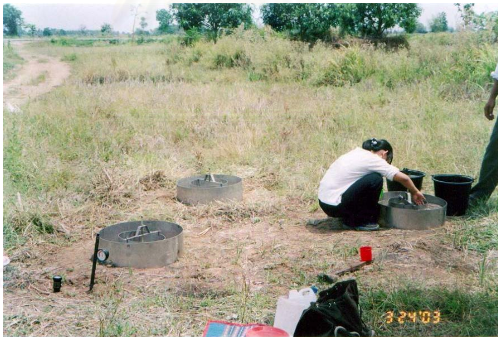
Figure 3.33 Double rings infiltrometers for testing the infiltration rate.
