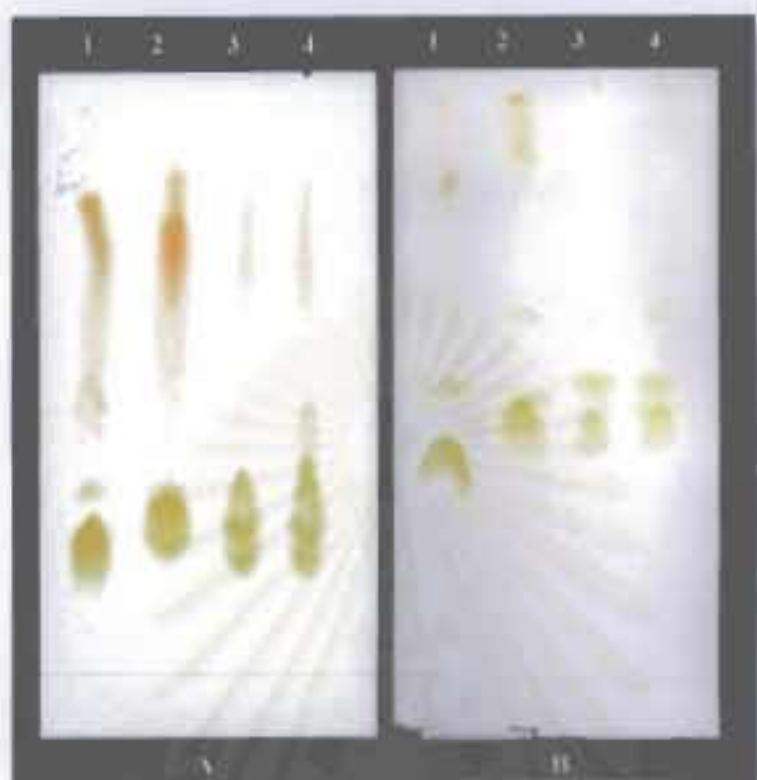
Figure 3.40 Separation of optical isomer of FDAA phenylalanine from E. coli BL21(DE3)pLysS contained pETPheDH on reversed phased TLC plates.
