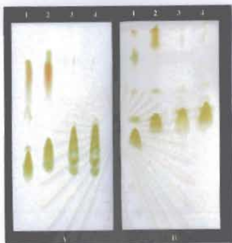
Figure 3.43 Separation of optical isomer of FDAA phenylalanine from E. coli BL21(DE3) contained pETFP on reversed phased TLC plates.
